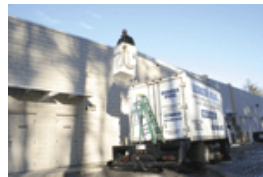
Steve Berger shows off the lift bucket on his truck, effectively eliminating the need to carry equipment and tools up and down ladders.
